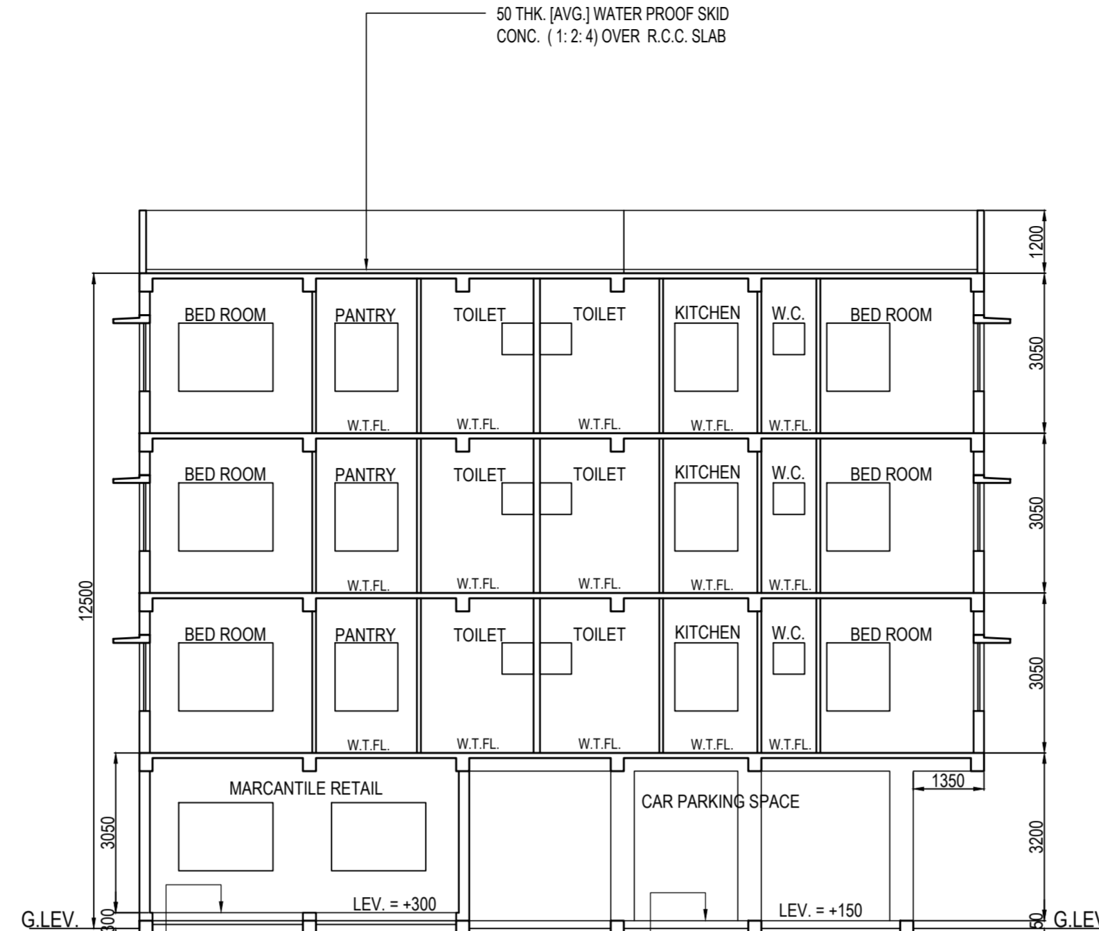
SECTION AT 'BB' SCALE = 1 : 100
